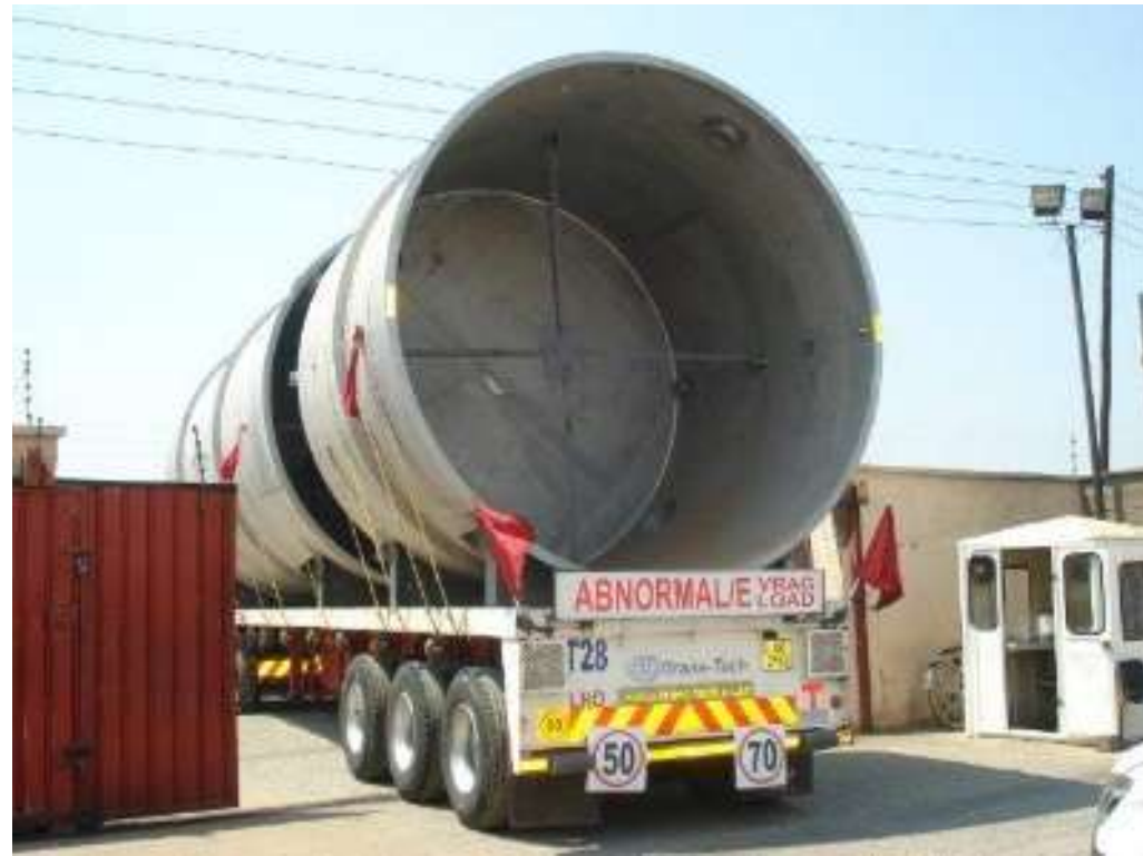
Tanks and skids transported by truck from South Africa to Kayelekera Mine in Malawi
